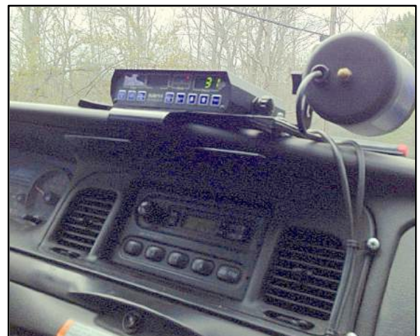
Moving radar monitors speed of cars approaching cruiser from both front and rear. Photo, J. Hauck, 2016.
