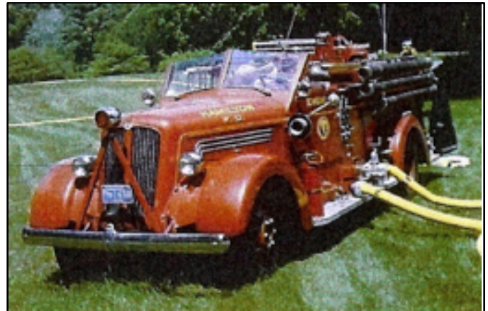
Engine 2, 1947 Seagrave , 750 gal., triple combination 50 gpm pumper, with open cab. Photo, Hamilton Fire Department
