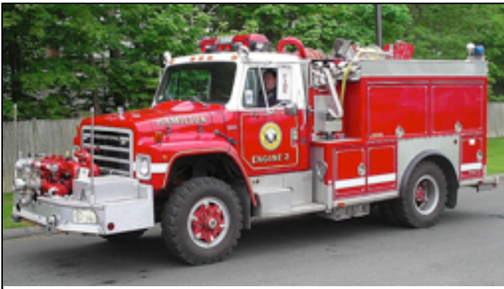
Engine 2, 1985, International Ranger , 1,000 gpm front mount pump, with a large diameter hose reel mounted in the back carrying 2,000 ft. of 4-in. hose. Photo, Hamilton Fire Department
