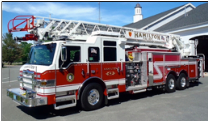
Ladder 4, 2014, Pierce Velocity , with 105-ft. aerial ladder and a 2,000 gpm/500 gal. tank. Photo, Hamilton Fire De-
