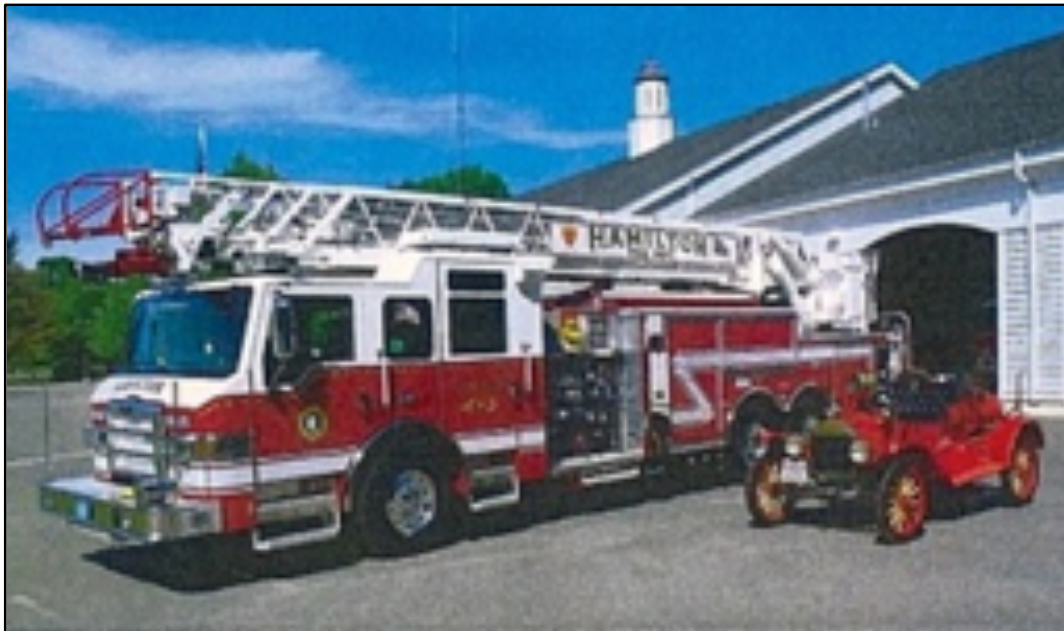
First apparatus , a 1916 American LaFrance triple combination chemical truck with a Ford model T chassis , in front of 2014 Pierce Velocity that is a pumper, has a water tank, fire hose, aerial ladder, and ground ladders. Photo, Hamilton Fire Department
