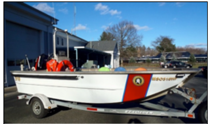
Boat, 1992 18-ft., run-about , with center-console and 90 hp outboard motor. Photo, Hamilton Fire Department
