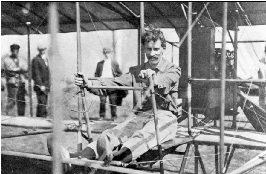
Augustus Herring, the pilot, used a hand-held steering rudder and foot-controlled elevating rudder. 25-hp engine and propeller, behind the pilot's seat, pushed the plane forward. Pushing a throttle pedal increased the engine to full power. Photo, Hamilton Historical Society.
