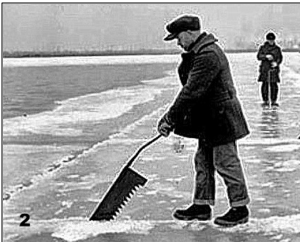
2 Using long saws , workers cut long floats of multiple ice cakes from the ice field. Photo Maine Maritime Museum
